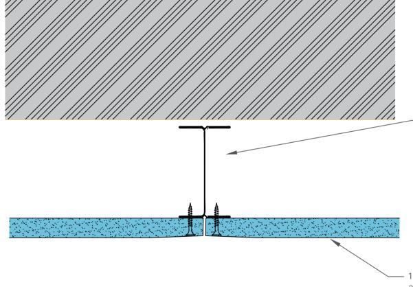
SPEEDLINE 70mm 'I' Studs at 600mm Ctrs
